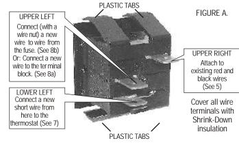
8b. On older units this wire may have gone directly to the fuse-holder. If so, cut the ring connector off the new wire. Strip back 1" of insulation on the old wire to the fuse-holder and the new wire. Twist the old and the new wire together. Screw the wire nut (supplied in the kit) tightly onto both wires to secure together. Tape the wire nut tightly with electrical tape. (See Figure A. UPPER LEFT)
